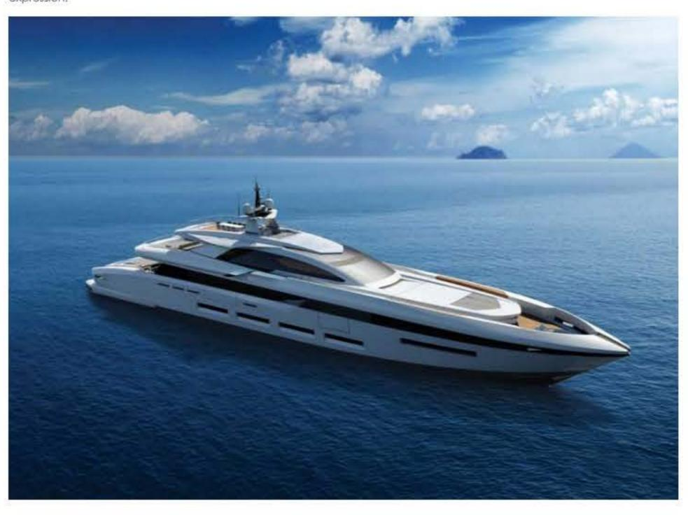
Length overall 58,00 mt (190,20') 2 x Kamewa Water Jet + Central booster Max beam 9,60 mt (31,49') Bow thruster Max draught 1.80 mt (5,90') Gyroscopic stabilizers
