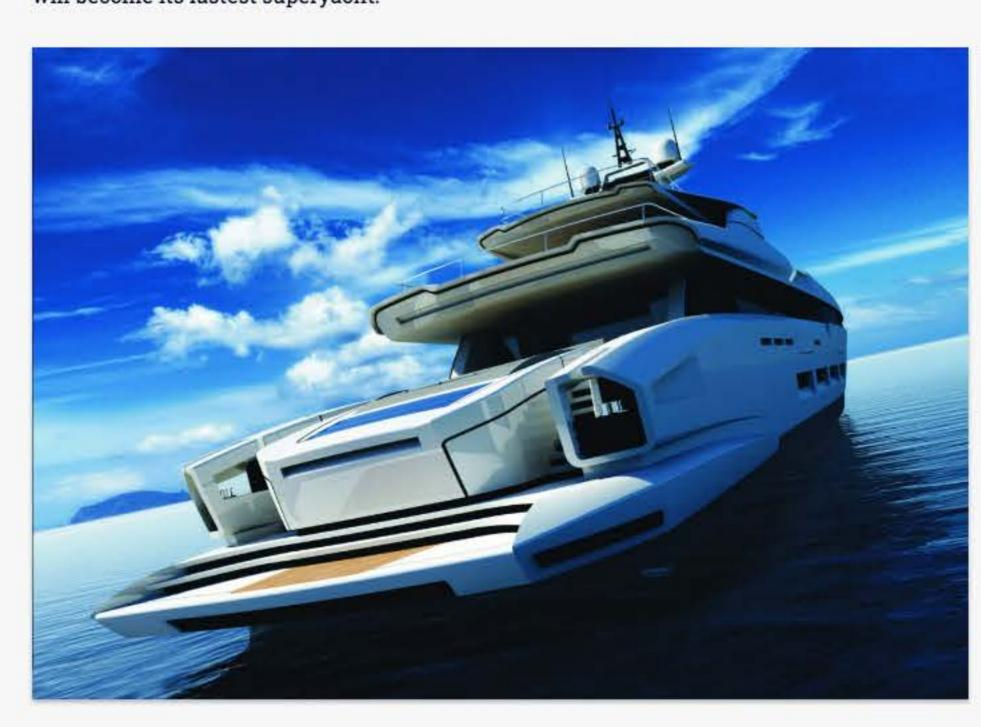
With a streamlined profile, the new concept oozes speed. The engine configuration confirms this with its triple engine setup: 3x 2,000 kW MTU diesel engines that drive twin Kamewa waterjets and a central booster. Top speed will be around 30 knots.
