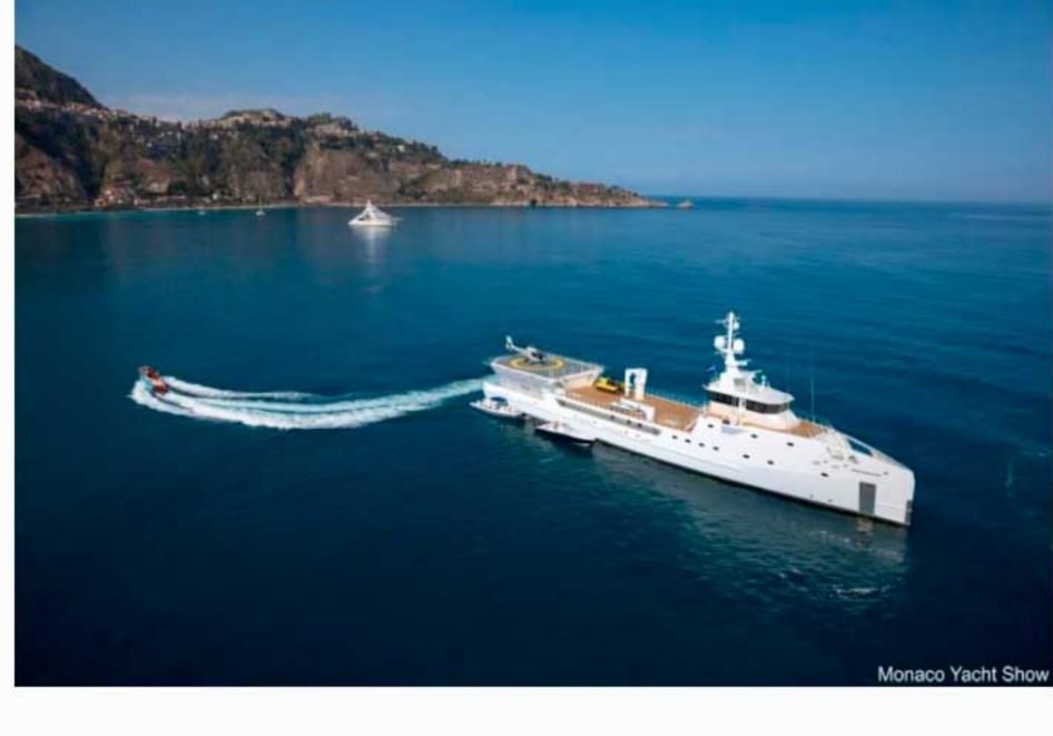
support vessel that made national headlines after it docked up next to the HMS Belfast on the Thames in May. It features 250 square metres of open deck space and its own helicopter landing pad and hangar. It is powered by four 3,000hp MTU 16V4000 M63L diesel engines, achieving a top speed of 20 knots and a cruising range of 4,500 nautical
