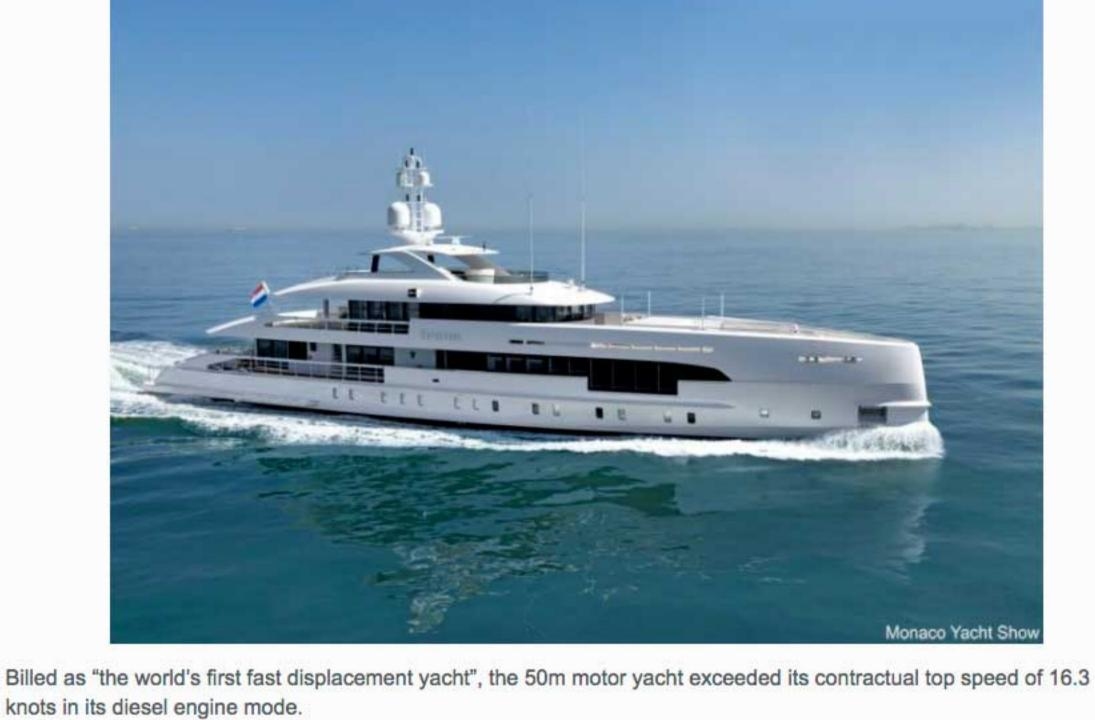
It also features a hybrid propulsion mode, powered by two 127kW water cooled motors, with a top speed of just over nine knots. The vessel's vertical bow, fixed swim platform and floor-to-ceiling glass windows present a unique profile. The architect is
